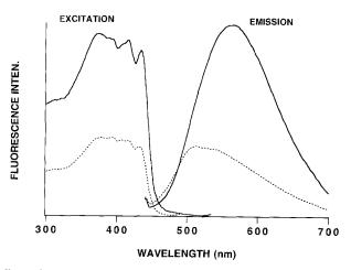
Figure 2 Fluorescence spectra of 30/70 PBO/AN film: ----, dried; annealed. Both emission spectra were excited at 430 nm, and excitation spectra were run at respective emission maxima
